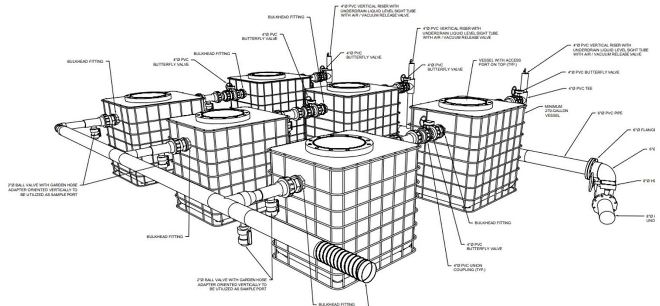
1 PHASE III UNDERDRAIN PFAS TREATMENT SYSTEM ISOMETRIC VIEW
